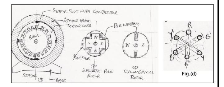
Fig. (b) represents the structure of a salient pole rotor where the poles are of projected type and are mounted on a spider and the field or the pole windings are wound over the pole core as shown.
