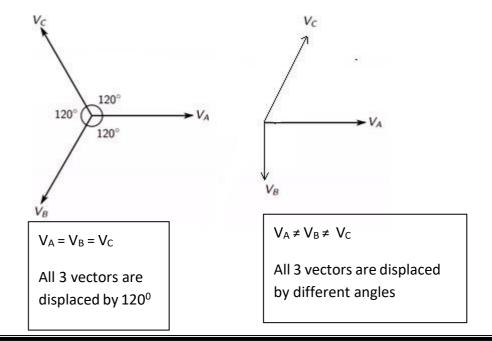
**Balanced load :** If the impedances in all the three phases are equal in magnitude then the load is said to be balanced .
