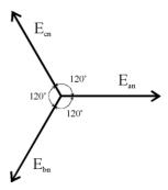
Stator conductors aa', bb' and cc' are mutually displaced by  $120^{0}$ . As the rotor rotates, the stator conductor cuts the flux and hence emf is induced in all 3 conductors.
